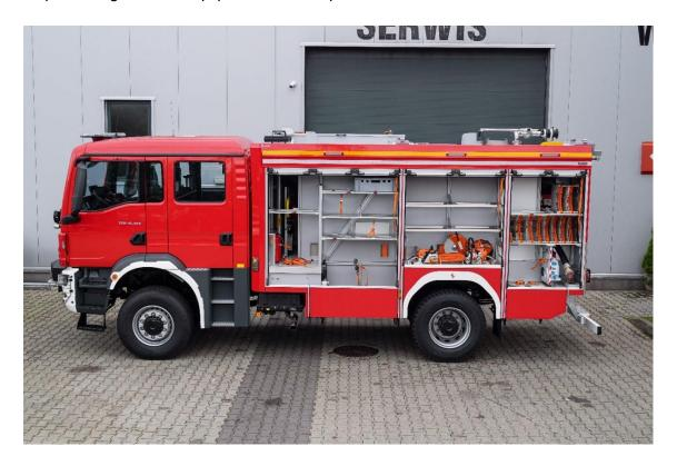
In the front part of the structure there is space for long elements that are often used during operations. There is a mount for medical equipment such as a stretcher, Kramer splints or a medical bag. The front compartment has a retractable panel with a mount for two Breahing Apparatus cameras and a drawer with a power generator.
