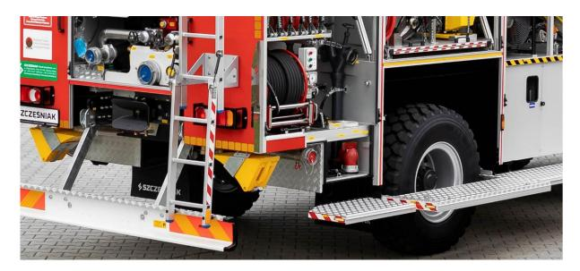
**Sprinkler system** installed in the chassis to limit chemical contamination zones or for fire-fighting purposes, equipped with 4 nozzles with a capacity of 50 dm <sup>3</sup>/min. each. Two sprinklers placed in front of the front axle, two sprinklers on the sides of the vehicle. Sprinklers are made of brass.
