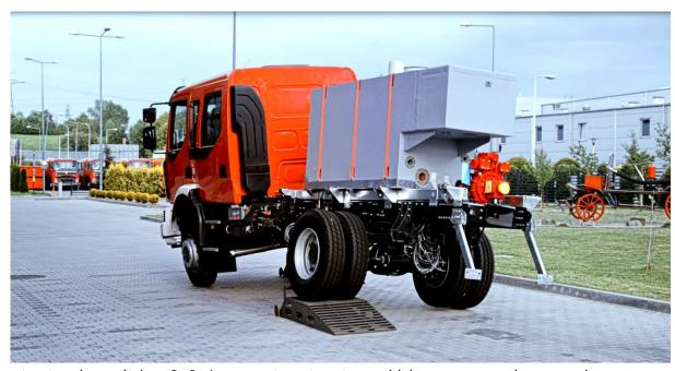
The structure is made in a 3+3+1 compartment system, which ensures maximum equipment capacity, ensuring a depth of 600 mm in each compartment.
