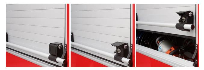
All equipment in superstructure are securely fastened by means of rattle-free fixings. Heavier equipment is fixed on telescopic runners or on sliding frames.
